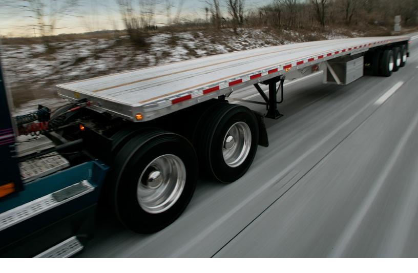
**BIG BUBBA FLATBED MODELS BOAST A GVWR OF 100,000 LBS.** and are rated at 70,000 lbs. in 10 feet and 60,000 lbs. in 4 feet — a legend that continues to set the standard for heavyweights. Not bad for a trailer that weighs an average of 3,000 lbs. less than any steel trailer even approaching Big Bubba's hauling capacity.
