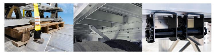
Multi-position tie down system offers flexibility to either tie down narrow loads to the center of the trailer or to the outside side rails.
